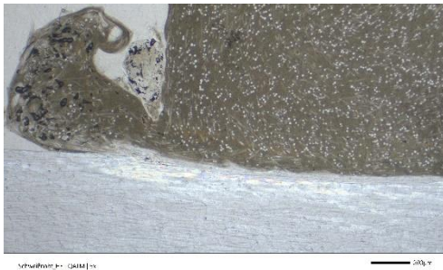
Thin section of a plastic weld seam transmitted light bright field.
